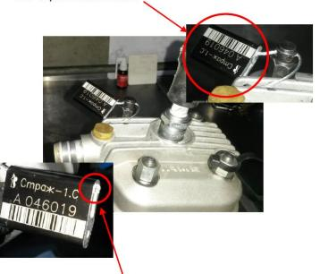
Don't forget to seal your engine and present your engine passport at the technical inspection.
